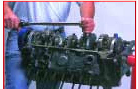
5. Using the instructions provided with the studs, tighten the nuts to proper torque values three times. NOTE: If using Loc-Tite or similar cement, proper preload must be achieved prior to it setting up.
